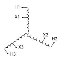
Three Phase Autotransformer with a capacity of 45kVA, transforming 277Y Volts to 115Y Volts
