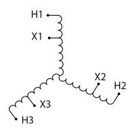
Three Phase Autotransformer with a capacity of 600kVA, transforming 347Y Volts to 110Y Volts
