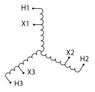
Three Phase Autotransformer with a capacity of 45kVA, transforming 277Y Volts to 480Y Volts
