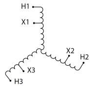
Three Phase Autotransformer with a capacity of 450kVA, transforming 347Y Volts to 110Y Volts
