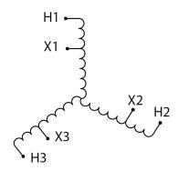
Three Phase Autotransformer with a capacity of 1500kVA, transforming 120Y Volts to 115Y Volts
