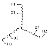
Three Phase Autotransformer with a capacity of 600kVA, transforming 480Y Volts to 240Y Volts
