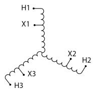
Three Phase Autotransformer with a capacity of 750kVA, transforming 600Y Volts to 400Y Volts
