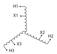
Three Phase Autotransformer with a capacity of 300kVA, transforming 240Y Volts to 220Y Volts
