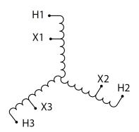
Three Phase Autotransformer with a capacity of 500kVA, transforming 440Y Volts to 110Y Volts
