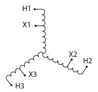
Three Phase Autotransformer with a capacity of 225kVA, transforming 200Y Volts to 575Y Volts
