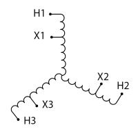
Three Phase Autotransformer with a capacity of 450kVA, transforming 400Y Volts to 460Y Volts
