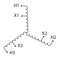
Three Phase Autotransformer with a capacity of 450kVA, transforming 415Y Volts to 110Y Volts
