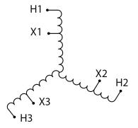
Three Phase Autotransformer with a capacity of 300kVA, transforming 277Y Volts to 480Y Volts
