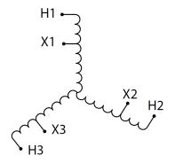
Three Phase Autotransformer with a capacity of 450kVA, transforming 416Y Volts to 120Y Volts
