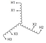
Three Phase Autotransformer with a capacity of 3kVA, transforming 277Y Volts to 110Y Volts
