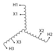
Three Phase Autotransformer with a capacity of 225kVA, transforming 220Y Volts to 347Y Volts
