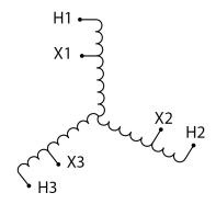
Three Phase Autotransformer with a capacity of 450kVA, transforming 440Y Volts to 400Y Volts
