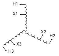
Three Phase Autotransformer with a capacity of 112.5kVA, transforming 115Y Volts to 415Y Volts
