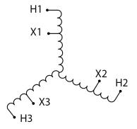
Three Phase Autotransformer with a capacity of 112.5kVA, transforming 120Y Volts to 575Y Volts
