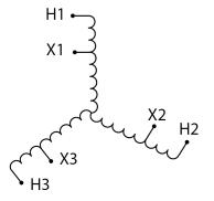
Three Phase Autotransformer with a capacity of 225kVA, transforming 240Y Volts to 460Y Volts
