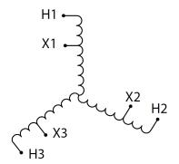
Three Phase Autotransformer with a capacity of 225kVA, transforming 240Y Volts to 460Y Volts
