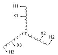
Three Phase Autotransformer with a capacity of 45kVA, transforming 480Y Volts to 208Y Volts
