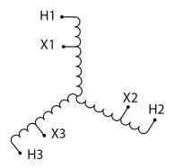
Three Phase Autotransformer with a capacity of 1000kVA, transforming 115Y Volts to 460Y Volts
