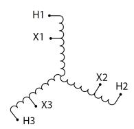
Three Phase Autotransformer with a capacity of 30kVA, transforming 380Y Volts to 110Y Volts
