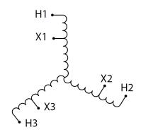
Three Phase Autotransformer with a capacity of 3kVA, transforming 380Y Volts to 220Y Volts
