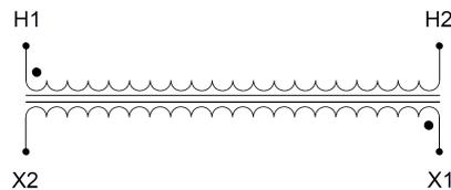
Single Phase Encapsulated Isolation Transformer with a capacity of 2kVA, transforming 460 Volts to 120/240 Volts
