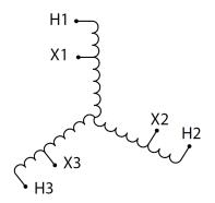
Three Phase Autotransformer with a capacity of 150kVA, transforming 220Y Volts to 120Y Volts
