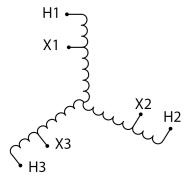
Three Phase Autotransformer with a capacity of 300kVA, transforming 460Y Volts to 220Y Volts
