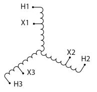
Three Phase Autotransformer with a capacity of 225kVA, transforming 347Y Volts to 200Y Volts
