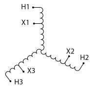
Three Phase Autotransformer with a capacity of 750kVA, transforming 120Y Volts to 240Y Volts
