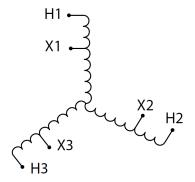
Three Phase Autotransformer with a capacity of 2500kVA, transforming 400Y Volts to 480Y Volts
