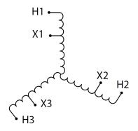
Three Phase Autotransformer with a capacity of 30kVA, transforming 575Y Volts to 120Y Volts
