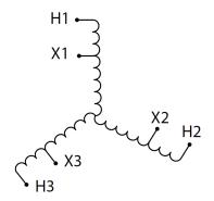
Three Phase Autotransformer with a capacity of 225kVA, transforming 440Y Volts to 575Y Volts
