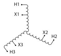
Three Phase Autotransformer with a capacity of 600kVA, transforming 120Y Volts to 416Y Volts
