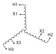
Three Phase Autotransformer with a capacity of 1000kVA, transforming 200Y Volts to 550Y Volts
