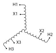
Three Phase Autotransformer with a capacity of 2500kVA, transforming 575Y Volts to 440Y Volts
