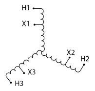
Three Phase Autotransformer with a capacity of 1000kVA, transforming 240Y Volts to 440Y Volts
