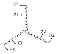
Three Phase Autotransformer with a capacity of 225kVA, transforming 550Y Volts to 380Y Volts
