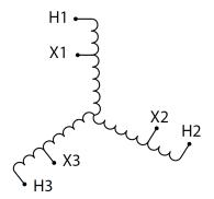
Three Phase Autotransformer with a capacity of 225kVA, transforming 550Y Volts to 208Y Volts
