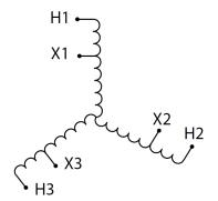
Three Phase Autotransformer with a capacity of 150kVA, transforming 380Y Volts to 230Y Volts
