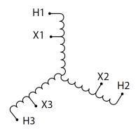
Three Phase Autotransformer with a capacity of 225kVA, transforming 575Y Volts to 380Y Volts
