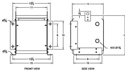
Single Phase Isolation Transformer with a capacity of 5kVA, transforming 220 Volts to 220/440 Volts
