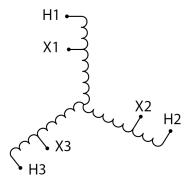
Three Phase Autotransformer with a capacity of 750kVA, transforming 200Y Volts to 400Y Volts
