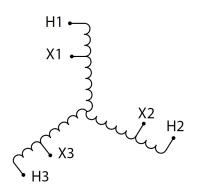
Three Phase Autotransformer with a capacity of 150kVA, transforming 415Y Volts to 200Y Volts
