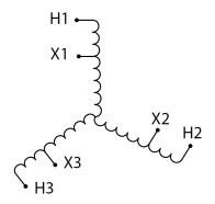
Three Phase Autotransformer with a capacity of 150kVA, transforming 416Y Volts to 220Y Volts
