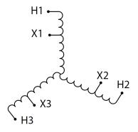
Three Phase Autotransformer with a capacity of 150kVA, transforming 440Y Volts to 380Y Volts
