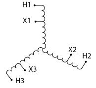
Three Phase Autotransformer with a capacity of 9kVA, transforming 277Y Volts to 600Y Volts
