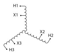
Three Phase Autotransformer with a capacity of 600kVA, transforming 208Y Volts to 600Y Volts
