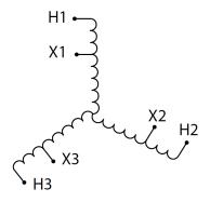
Three Phase Autotransformer with a capacity of 112.5kVA, transforming 415Y Volts to 347Y Volts
