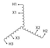
Three Phase Autotransformer with a capacity of 112.5kVA, transforming 415Y Volts to 230Y Volts
